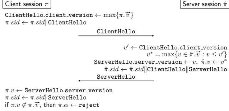
Figure 2:  $\text{NP}_v$ : No-fallback version negotiation protocol in standard TLS
