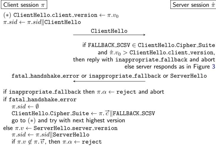
Figure 4:  $\text{NP}_{v\text{-fb-scsv}}$ : Fallback negotiation in TLS with signalling ciphersuite value
