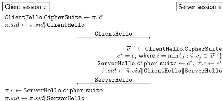
Figure 1: NP<sub>CS</sub>: Ciphersuite negotiation protocol in TLS
